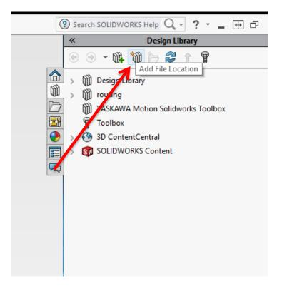
Step 4: Input the location on your computer where the "YASKAWA Motion Solidworks Toolbox VX.XX" was stored
