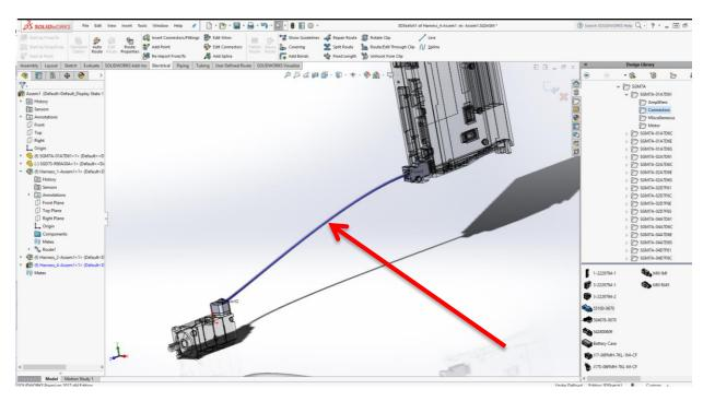
Step 2: Click the edit wires button on the Electrical Routing Tab
